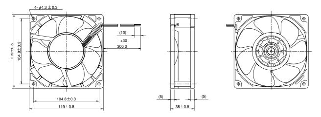
Fig. 4: Dimensions of the Oil Proof Fan, "San Ace 120WF"
