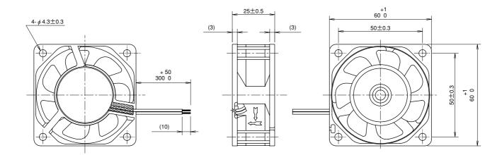
Fig. 3: Dimensions of the Oil Proof Fan, "San Ace 60WF"
