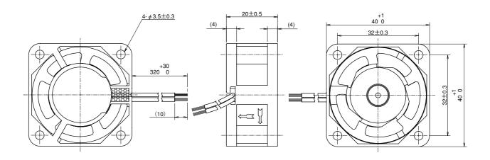
Fig. 2: Dimensions of the Oil Proof Fan, "San Ace 40WF"
